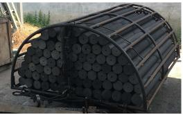
to form parallel structures that slide easily against one another. This is where the slippery feeling of graphite comes from. After a 3-4 week heating and cooling process, the carbon rods have been fully converted to a graphite rod.
